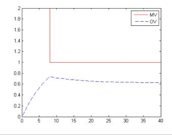
Evaluate a scenario at a single time instance, plotting the predicted optimal MV and OV sequences over the prediction horizon.
