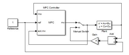
Do not connect this option to leave the ext.mv inport unconnected. In either case, the model predictive controller assumes that the plant uses the MV signals sent by the MPC Controller block. In the preceding example, the external MV signal always provides the model predictive controller that the control signal actually used in the plant. Otherwise, the model predictive controller's internal state estimate would be inaccurate.
